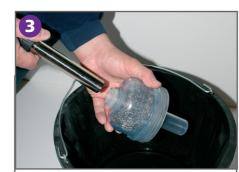
Once removed, place the clear base over a bucket. Unscrew and remove the magnet cap and rinse the sheath.
